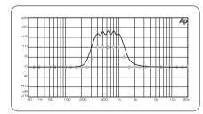
Graphic equalizer without frequency response correction (UNCORRECTED)
